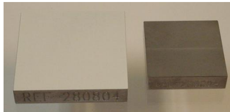
Figure 3.4 Reference Plane and Calibration Blocks
