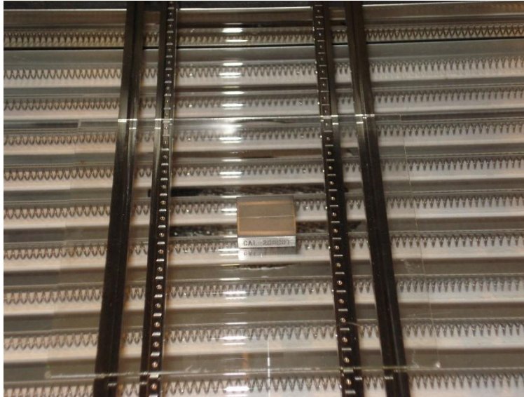
Figure 3.11 Calibration Block in the Oven
